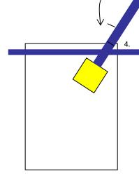
Return the sponge part of the Sponge to the sterile sample bag. Do not insert the handle past the thumbstop. Break off the handle by holding the sponge in place from outside the bag and bending the handle back and forth at the point where it joins onto the sponge (do not try to break at thumbstop). The sponge will drop to the bottom of the bag.
