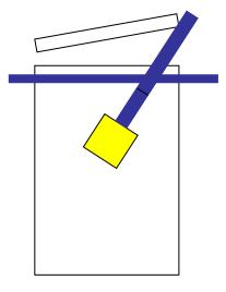
Tear open the bag along the perforation. Feed the Sponge handle through the opening, by pushing up from outside the bag. Grasp the handle above the thumbstop and remove the Sponge from the bag. To avoid contamination do not touch the space between the thumbstop and sponge, or the sponge itself.
