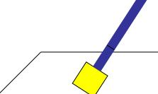
Using both sides of the sponge swab the surface back and forth for a period of approximately 30 seconds. If a template is being used swab in all directions within the template area.
