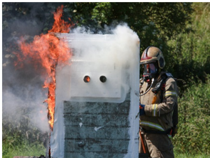
Checkmate - Demonstrating a burning panel with and without fire stopping products
